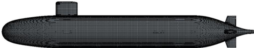
Figure. 5. The surface mesh of the underwater vehicle.
