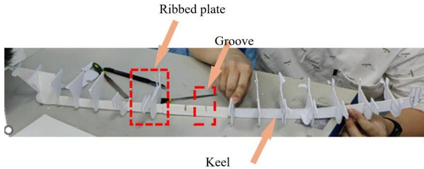
**Figure. 9.** Hull frame.
