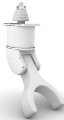
Figure. 4. Sacrificial anode inspection device.
